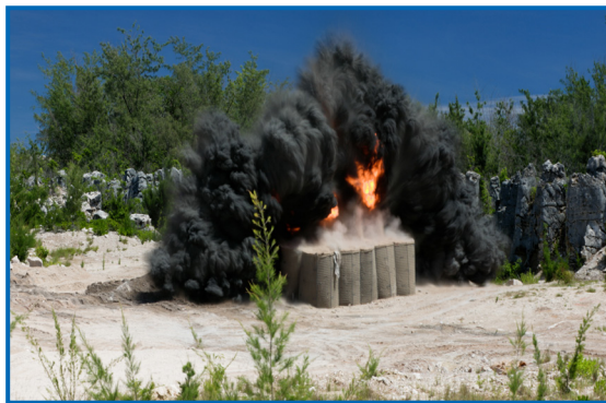
The 500lb aircraft UXO is buried under dirt reinforced with hesco barriers for detonation at Topside on 20 July
